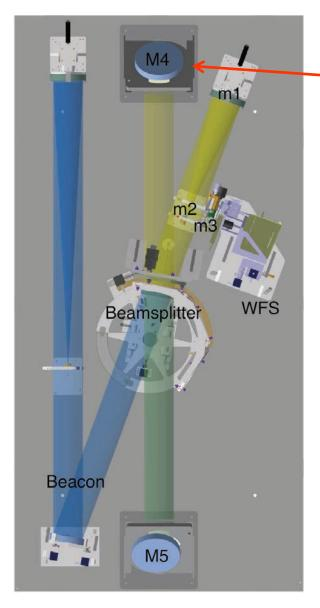
Phase II funds replacing M4 with a deformable mirror at each telescope which will enable us to correct for atmospheric seeing and increase scientific throughput.
